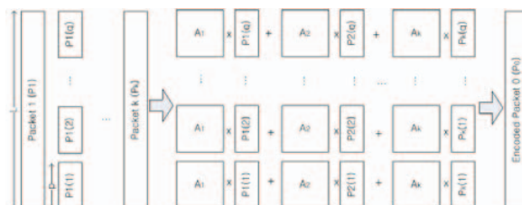
Fig. 1. Encoding process of matrix network coding.
